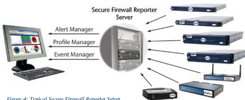
Figure 4: Typical Secure Firewall Reporter Setup
