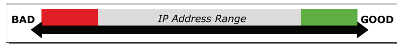
Figure 3: First-generation reputation systems assigned senders either a “bad” or “good” rating based on inaccurate and anecdotal blacklists and whitelists. IP addresses that should have fallen somewhere in the middle were left for an administrator to manually determine, potentially leading to incorrect classification.
